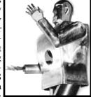
composed of 48 telephone relays (though this number may have varied over time) and the control logic was reportedly to count the number of distinct syllables in a command as a trigger to start the corresponding pre-canned actions.
